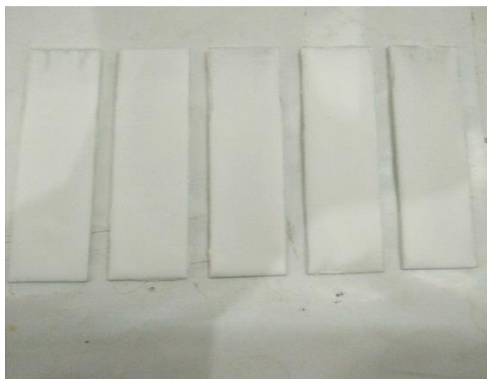
Fig 3.1 Prepared TLC Plate
