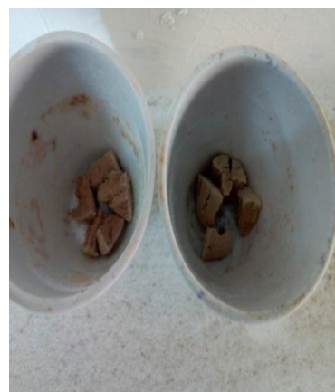
(vi) After calcinations at 750 °C
