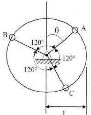
2(b) The three forces shown and a couple of magnitude M = 100 N-m are applied to the 17 angle bracket. (i) Find the resultant of this system of forces (ii) Locate the points where the line of action of the resultant intersects line AB and line BC.
