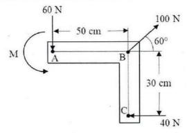
3(a) Two rods are welded together to form a T-shaped lever which is acted upon by a 680 N force as shown. Determine the moment of the force about rod AB.
