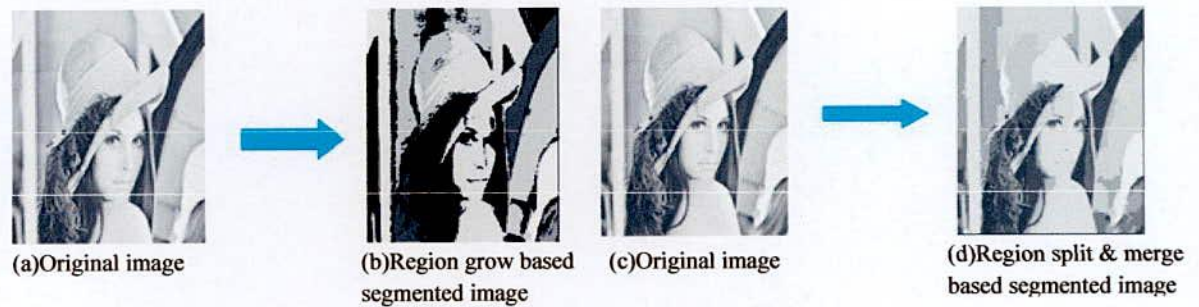
Figure 4.3: Comparison of Region growing and Region split & Merge segmentation process
