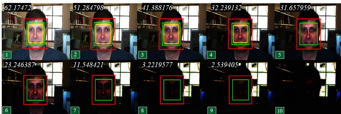
Figure 4.2: Observation of the behavior of HFFD-RGB and HFFD-S-RGB-R on a sample image by gradually darkening it (none of them can detect face when light intensity is less than 2.539405).
