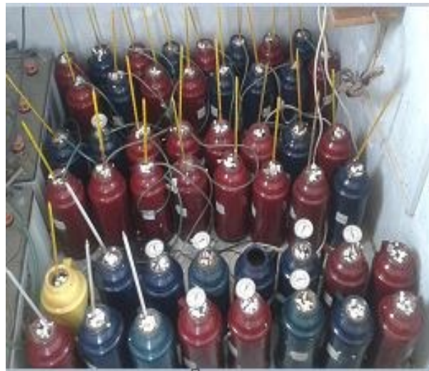
Figure 3.8: Experimental setup for the determination of volatile solids degradation.
