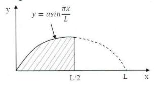
6(a) Determine by direct integration the moment of inertia and radius of gyration of the 17 shaded area as shown with respect to x-axis.
