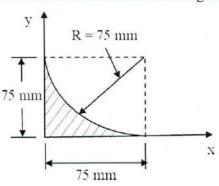
5(b) Determine by direct integration the centroid of the area shown in figure.
