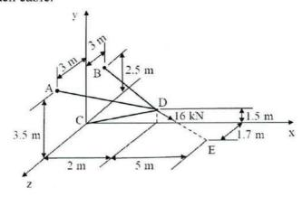
2(b) Two forces are applied to the vertical pole as shown in figure. Determine the 17 components of the forces and couple at O equivalent to the two-force system.
