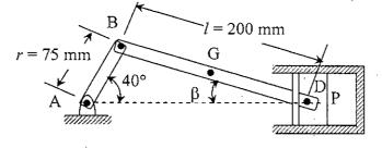
5(b) Two rotating rods connected by slider block P. Two rods attached at A rotates with a constant angular velocity  $\omega_{\Lambda}$ . For the given data, determine for the position shown (i) the angular velocity of the rod attached at B, (ii) the relative velocity of the slider block P with respect to the rod on which it slides. Given, b = 20 cm,  $\omega_{\Lambda} = 6$  rad/sec.
