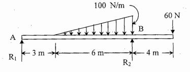
6(a) Find the relation R and the moment at the wall for the propped beam as shown in figure. 18
