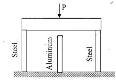
2(b) A rigid bar of negligible weight is supported as shown in figure. If W = 80 kN, compute 18 the temperature change that will cause the stress in the steel rod to be 55 MPa.
