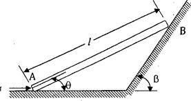
6(a) End A of rod AB moves to the right with a constant velocity of 2.5 m/sec. For the position 18 shown, determine (i) the angular acceleration of rod AB, and (ii) the acceleration of the midpoint G of rod AB.
