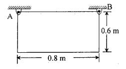
7(a) Two disk A and B of mass  $m_A = 2.8$  kg and  $m_B = 5$  kg are connected by a belt as shown. 17 Assuming no sliping between the belt and the disks, determine the angular acceleration of each disc if a 4 Nm couple M is applied to disk A.
