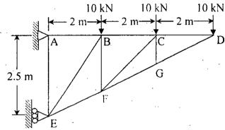
4(b) Determine the components of all forces acting on each member of the frame shown in figure.
