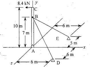
Determine the forces in each member of the truss shown in figure. 4(a)
