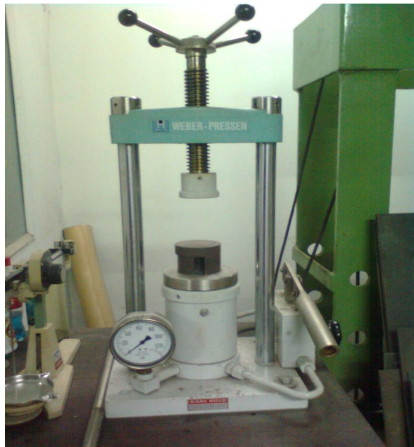
Figure 3.3 Hydraulic press used to make different shaped samples.
