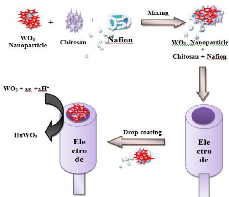
Figure 4.7: Schematic diagram of stepwise fabrication of the pH sensor
