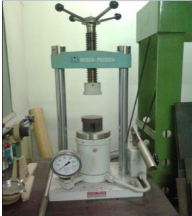
Figure 3.4: Hydraulic press used to make different shaped samples.
