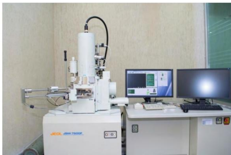
Figure 3.10: Field Emission Scanning Electron Microscope (FESEM).
