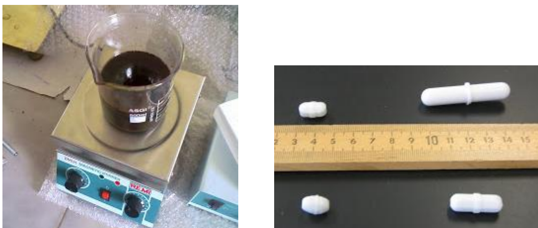
Figure 3.1: Magnetic stirring with hot pot and beaker and magnetic bars in different size
