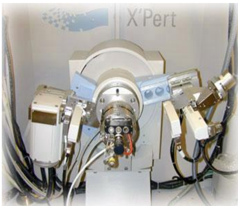
Figure 3.10: Internal arrangement of a PHILIPS X' Pert PRO X-ray diffractometer
