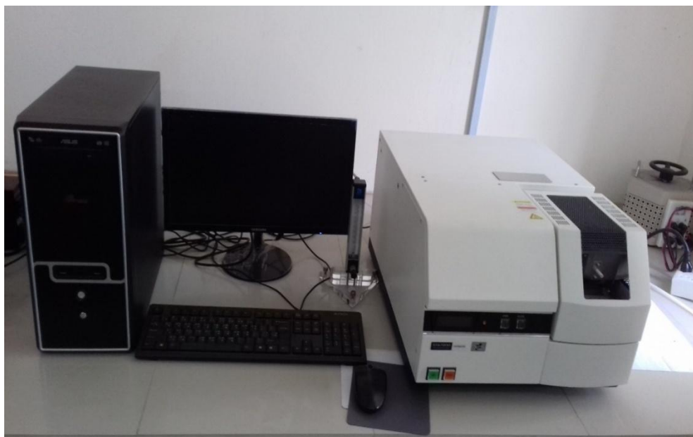
Figure 3.7: TA7000 Series Simultaneous Thermogravimetric Analyzer
