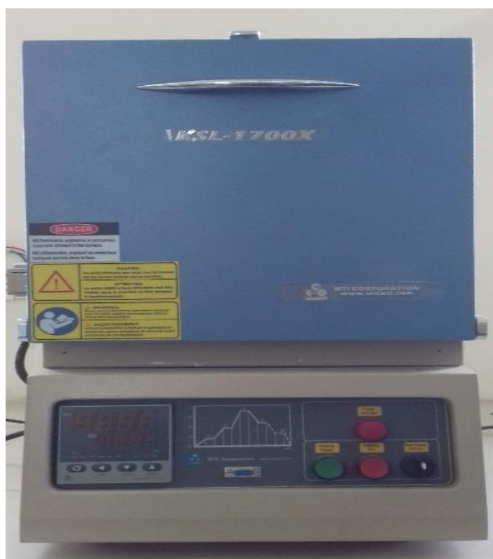
Figure 3.8: MTI - KSL-1700X-S High Temperature Muffle Furnaces
