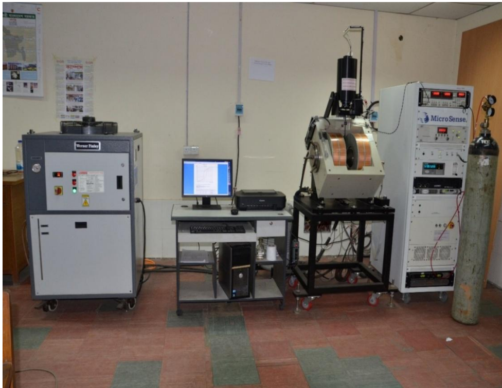
Figure 3.12: Vibrating Sample Magnetometer at Materials Science Division, AECD
