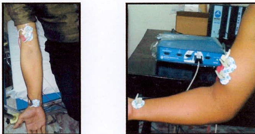
Figure 5.4: Electrode placement and lead setting arrangement along Biceps Brachii of subjects.
