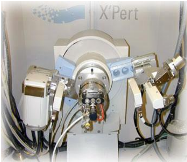
Figure 3.7: Internal arrangement of a PHILIPS X' Pert PRO X-ray diffractometer
