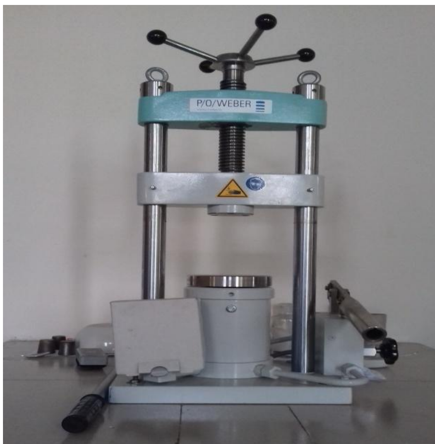
Figure 3.2: Hydraulic press used to make different shaped samples
