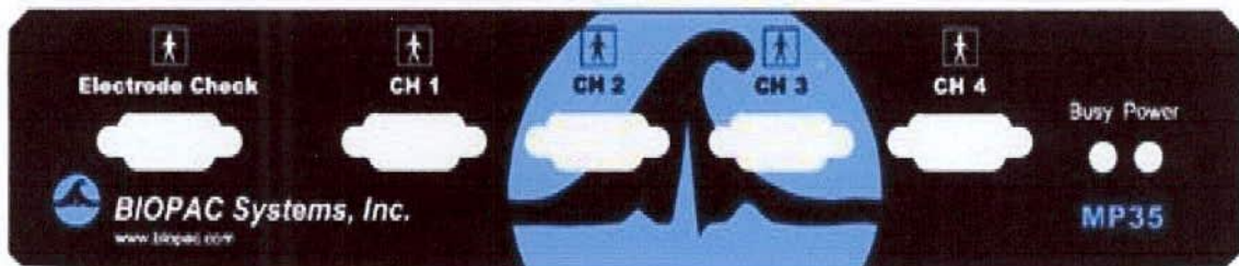
Figure 3.3 The front panel of the MP3X has an electrode check port, four analog input ports, and two status indicators. Input ports: CH 1, CH 2, CH 3, and CH 4
