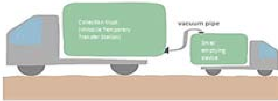
Figure 5.5: Mobile Secondary Transfer Station (Source: Dgroup Discussion of SNV, 2015)
