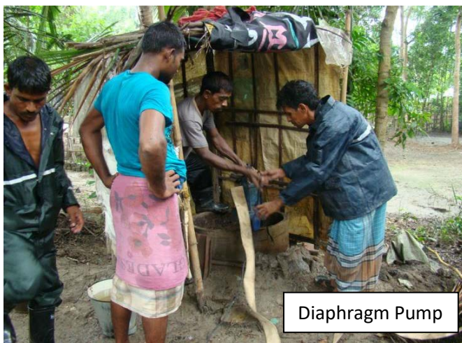
Figure 5.3: Small emptying devices (Source: BRAC report, 2015)
