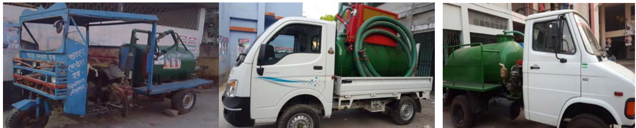
Figure 4.32: Vacutug of Jhenaidah Municipality
