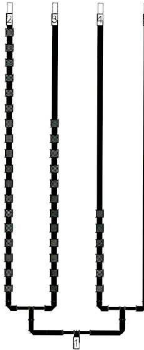
Fig. 7.3: Geometry of a 4 by 1 feed network assisted by 18 square patterned PBG elements with FF of 0.5. The geometry is developed in MGRID of IE 3D on substrate having dielectric constant of 2.46 and height of 31 mils.
