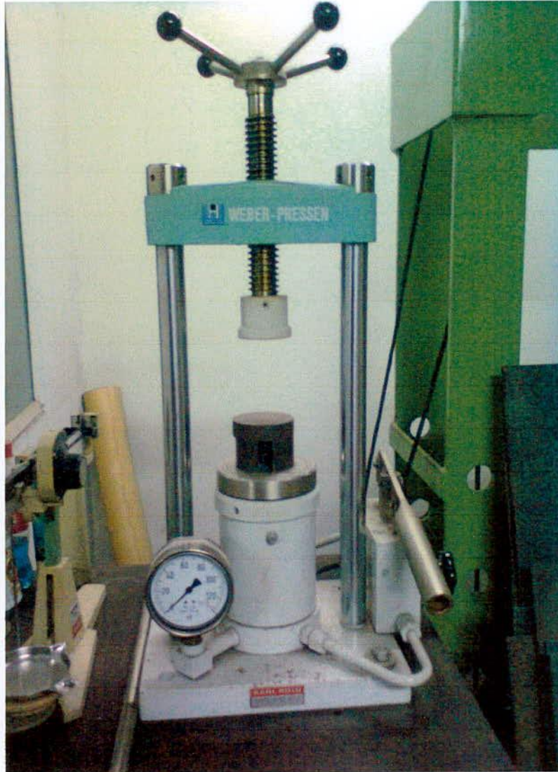
Fig. 3.3 Hydraulic press used to make different shaped samples
