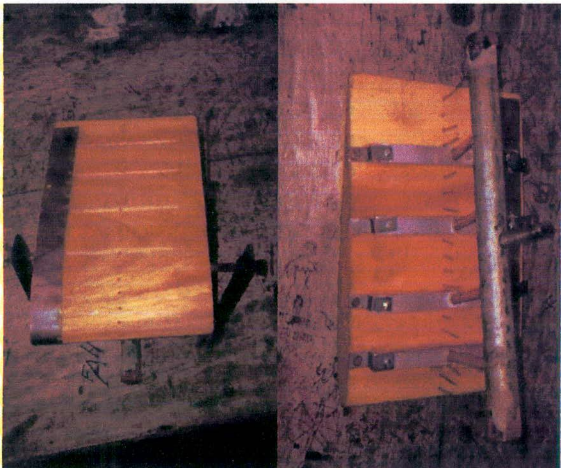
Figure 4.3(a): Construction of Model NACA 2415 with four slots
