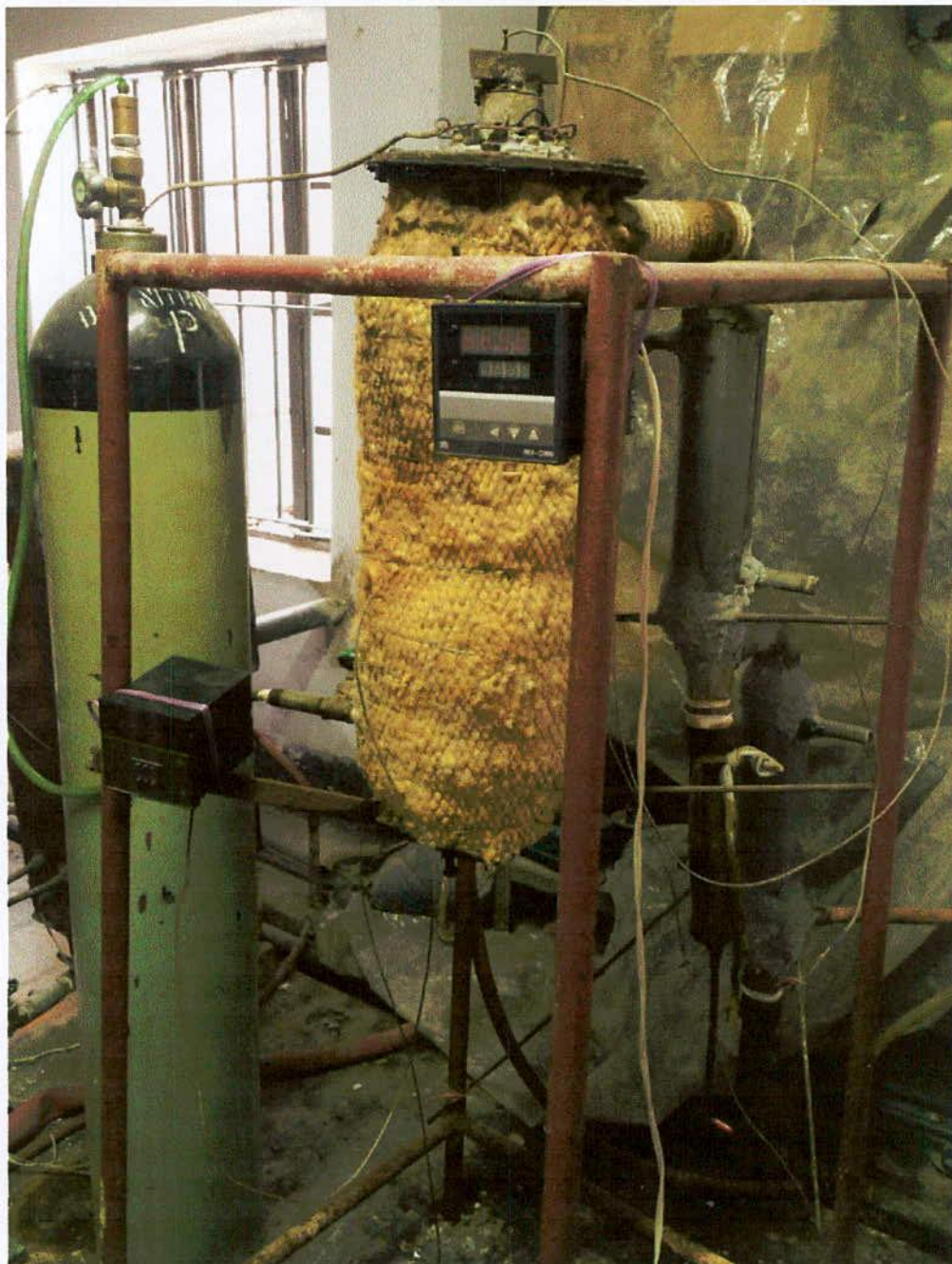
Figure 3.4: Photograph of the fixed-bed fire-tube heating pyrolysis system
