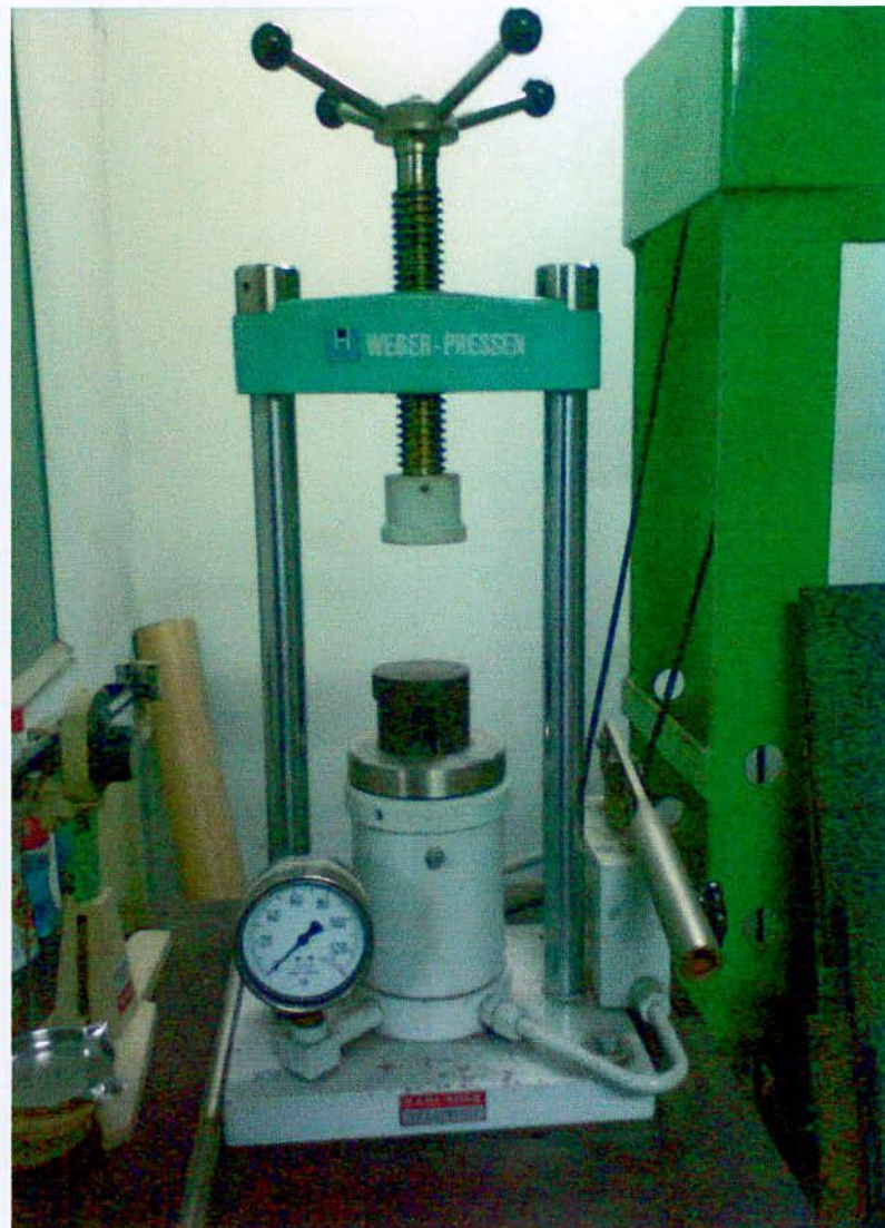
Fig. 3.2 Hydraulic press used to make different shaped samples
