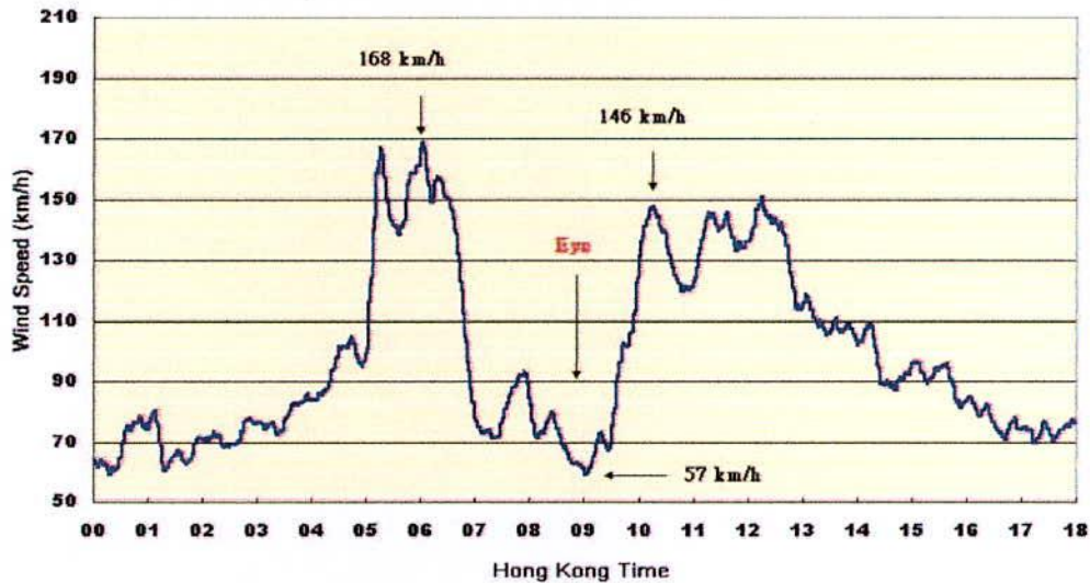
Figure 2.5 Wind speed record of Waglan Island during the direct hit of Typhoon York over Hong Kong on 16 September 1999. Notice the dramatic fall and rise in wind strength during the passage of the eye of York [44].
