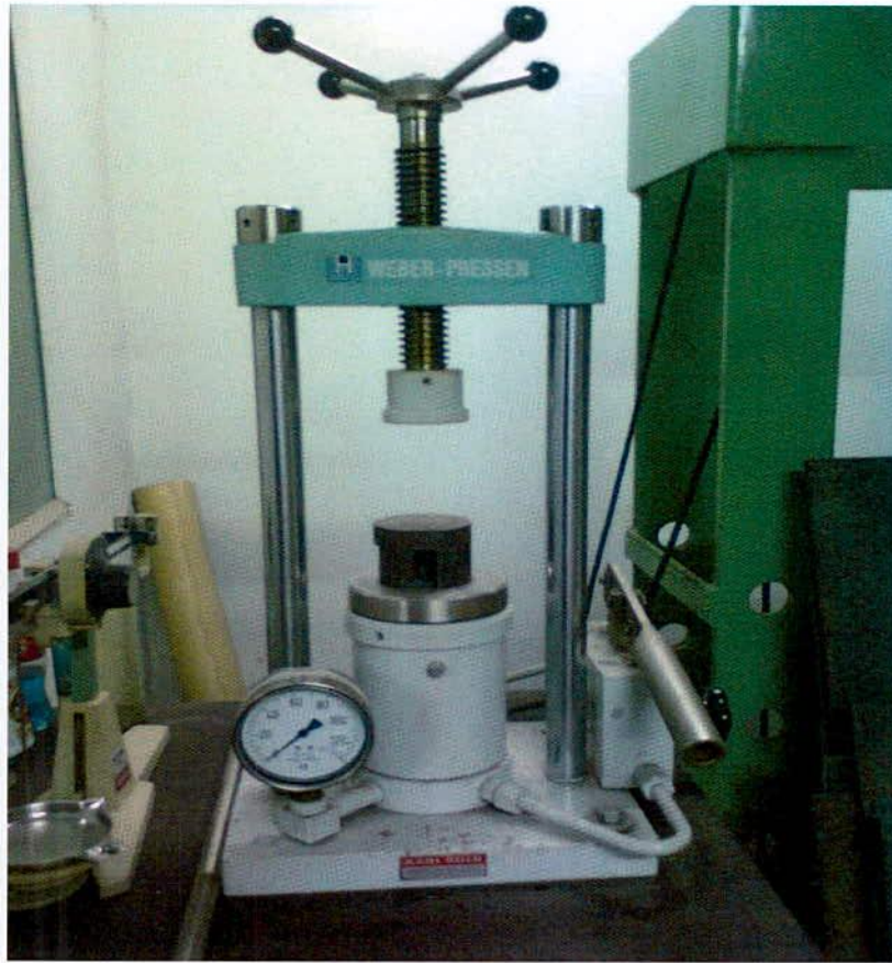
Fig.3.2 Hydraulic press used to make different shaped samples.
