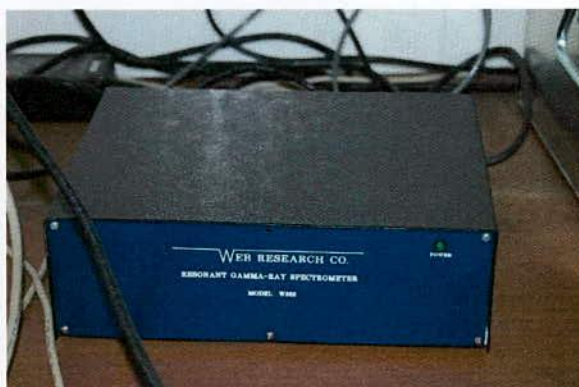
Fig. 3.16 SEE Co. MS4 Spectrometer recording a Mossbauer spectrum
