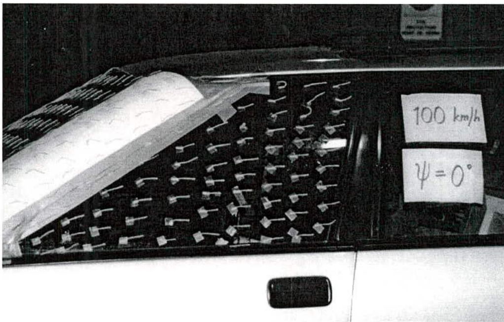
Figure 4.5: Side View of Flow Visualisation with Modified A-pillar, Yaw = 0^\circ , Speed = 100 km/h
