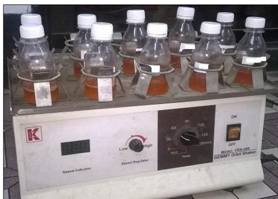
Figure 3.6.8 Bottles were placed in shaker to study the contact time.
