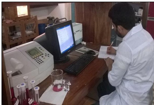
Figure 3.6.7 taking absorbance of different concentrated solution of dyes
