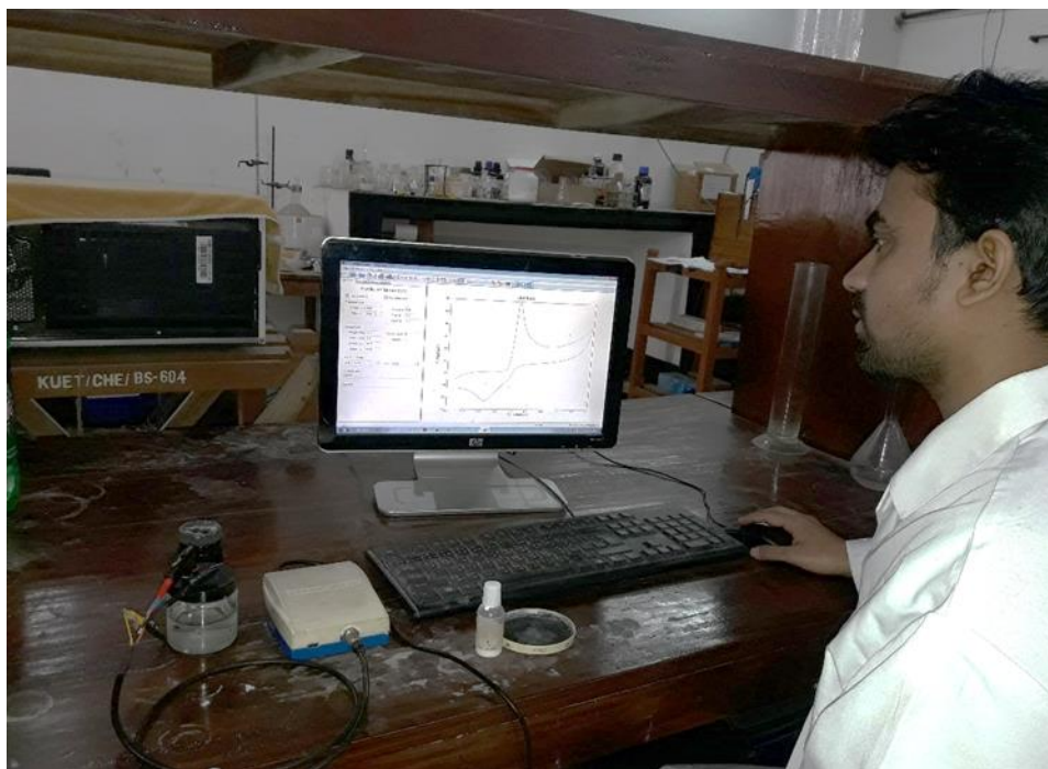
Figure 3.9: Experimental setup (Software controlled Potentiostat ( \mu stat 400))
