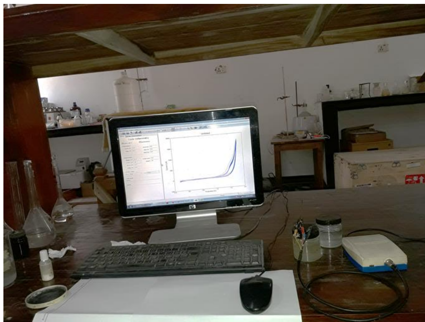
Figure 3.3: The computer controlled potentiostat ( \mu Stat 400, DropSens)
