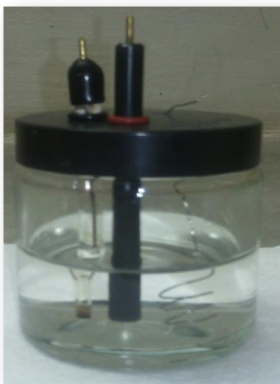
Figure 3.3: The three electrode system consisting of a working electrode, a reference electrode and a counter electrode.
