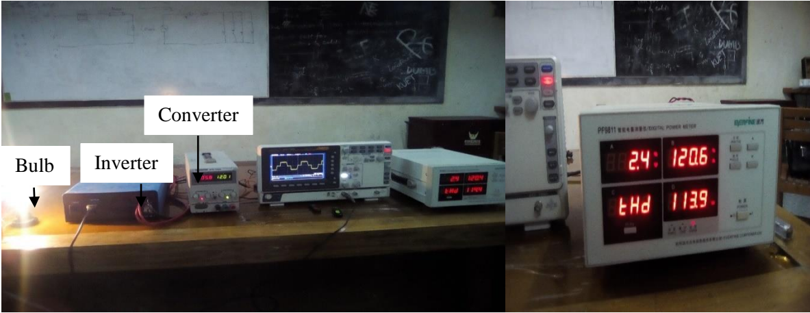
Figure 4.4: Total setup of harmonic analysis of a line supplied inverter with converter and load.
