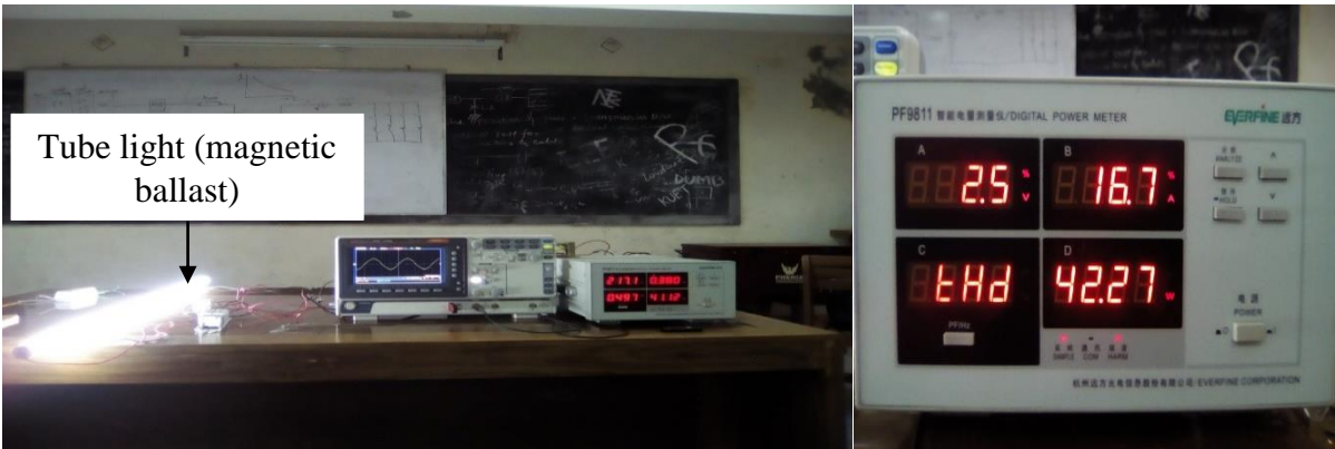
Figure 4.1: Total setup of the harmonic analysis of a tube light (magnetic ballast).
