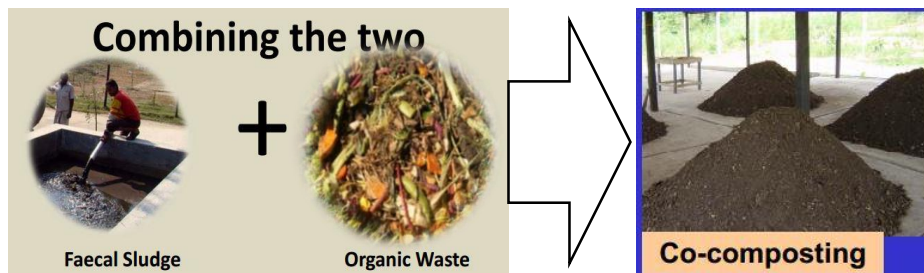
Figure 4.6: Co-composting of Faecal Sludge and Organic Solid Waste
