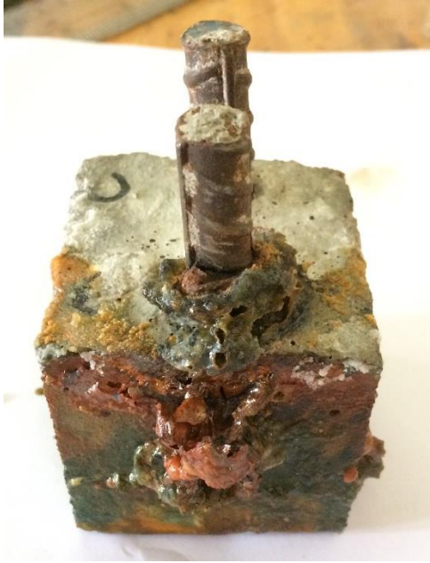
Figure 6.6: Steel and Zinc Anode after Test
