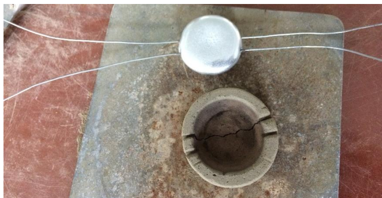
Figure 6.1: Preparation of Zinc Anode
