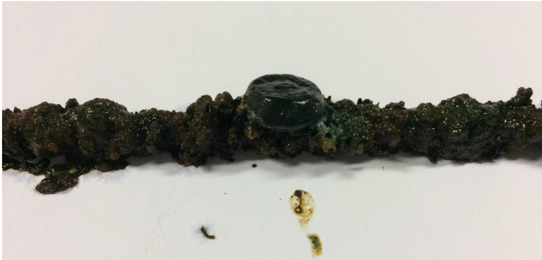
Figure 6.7: Steel and Zinc Anode after Test for Corroding Surface Area of 11300 mm 2
