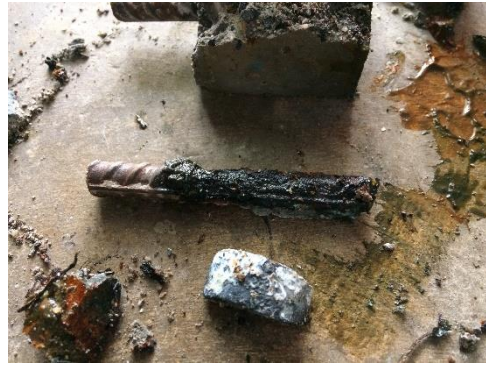
Figure 6.6: Steel and Zinc Anode after Test
