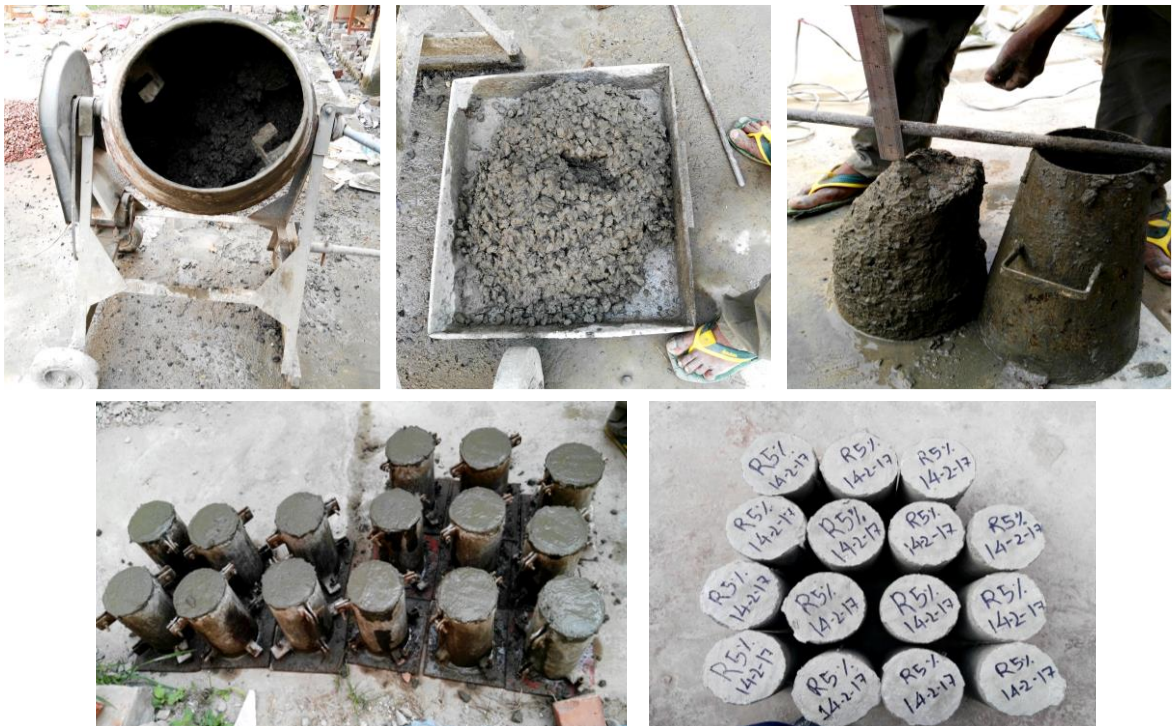
Figure 3.6: Preparation of cylindrical concrete specimens for compressive strength test.
