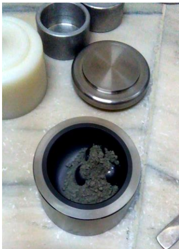
d. Hand grinding was done to produce cement or CW powder and cellulose mixed powder.
