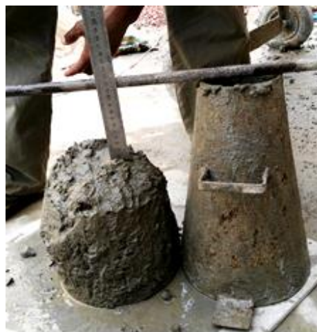
Figure 4.4: Slump value measurement.
