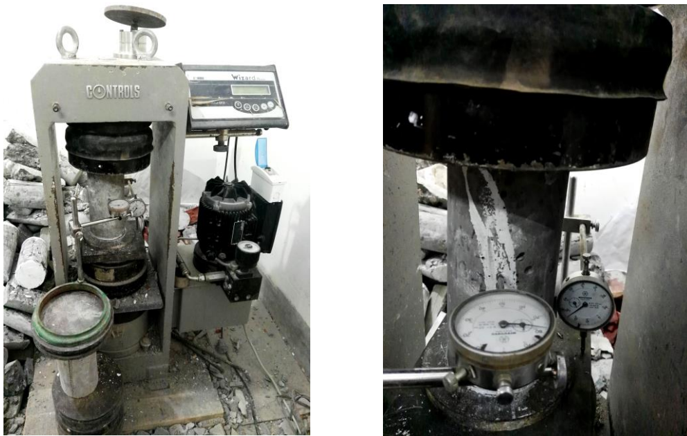
Figure 3.8: Compressive strength test setup of cylindrical concrete specimens.
