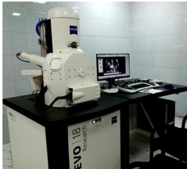
Figure 3.15: The scanning electron microscope SEM of type EVO 18 Research (Photo taken by author).
