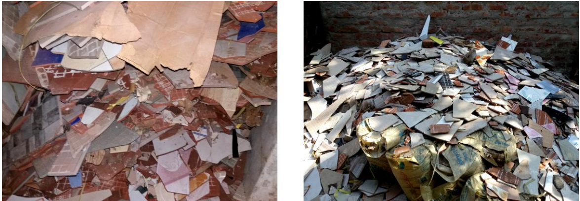
Figure 3.2: Field photo of waste ceramic tiles (white and red mixed).
