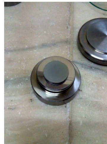
f. Placed the grinded powder in a sample holder and weighted.
