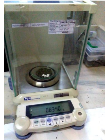
c. Cellulose binder was mixed with CW powder (0.80~0.85 gm).
