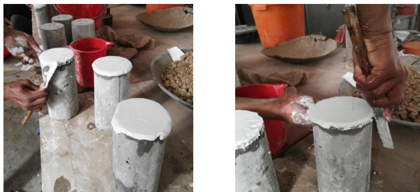
Figure 3.7: Gypsum capping of cylindrical concrete specimens.
