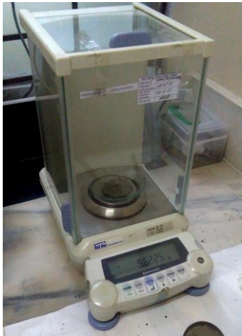
a. Weighted the cement or CW powder ~ 10 gm.
