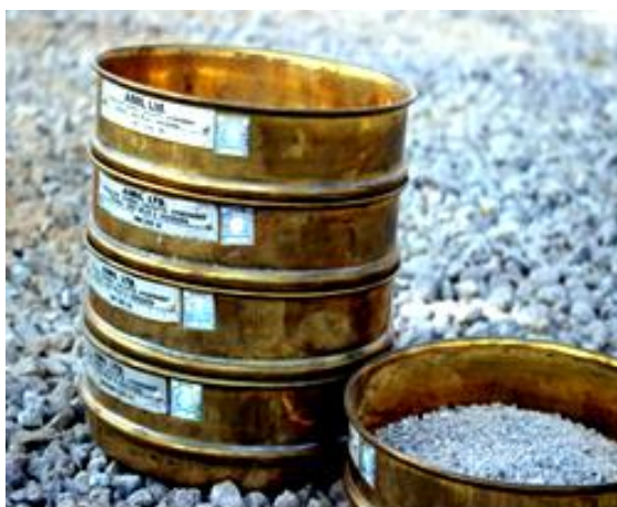
Figure 3.5: Sieve analysis technique.
