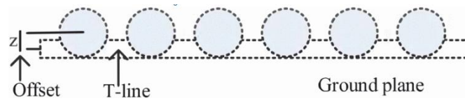
Fig 2.7. Offset in uniform EBGs assisted T-line [67]
