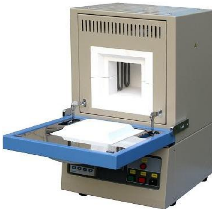
Figure 3.5: High Temperature Muffle Furnace (KSL-1700X-S) at Solid State Physics Laboratory, KUET
