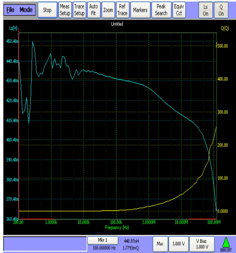
Figure 3.14: Complex permeability measurement by Wayne Kerr Precision Impedance analyzer
