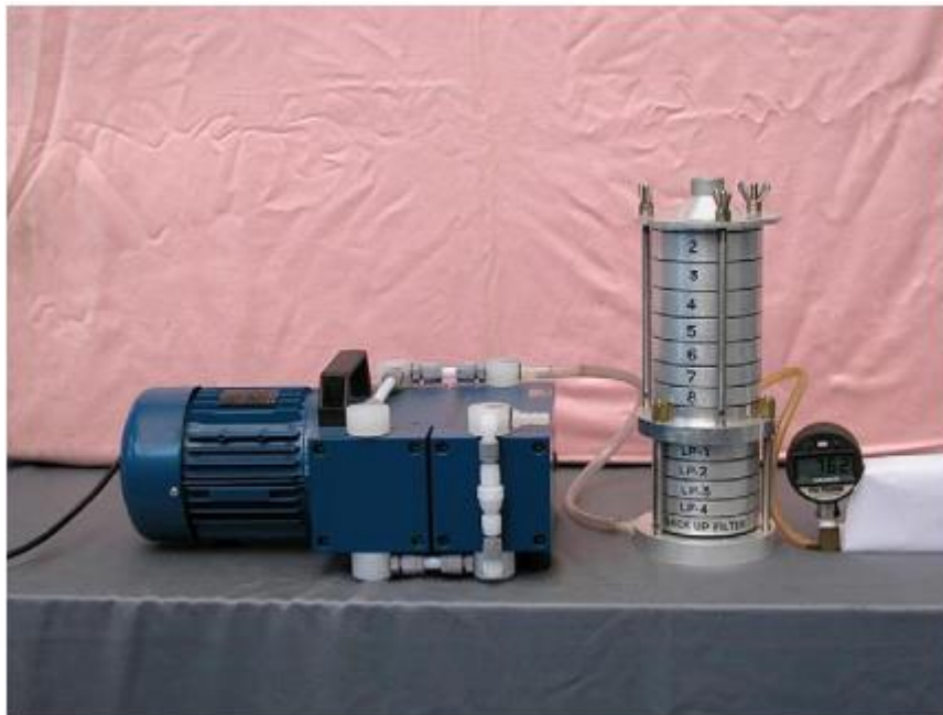
Figure 2-14 A variable configuration cascade impactor (VCCI) developed by Singh et. al. , 2010
