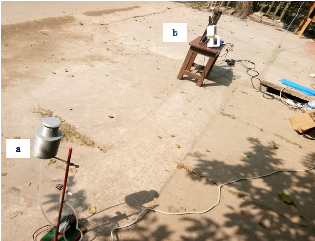
Figure 3-8 The field experimental setup of (a) designed sampler (b) standard reference sampler
