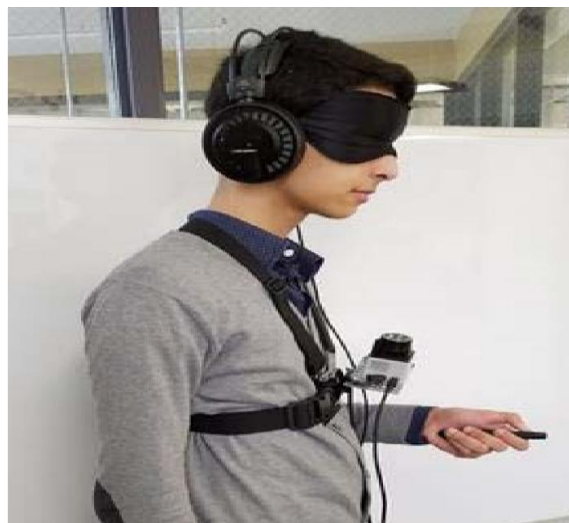
Figure 2.11: Participants wearing the LIDAR assist spatial sensing system and equipped with a laser pointer [58] .
