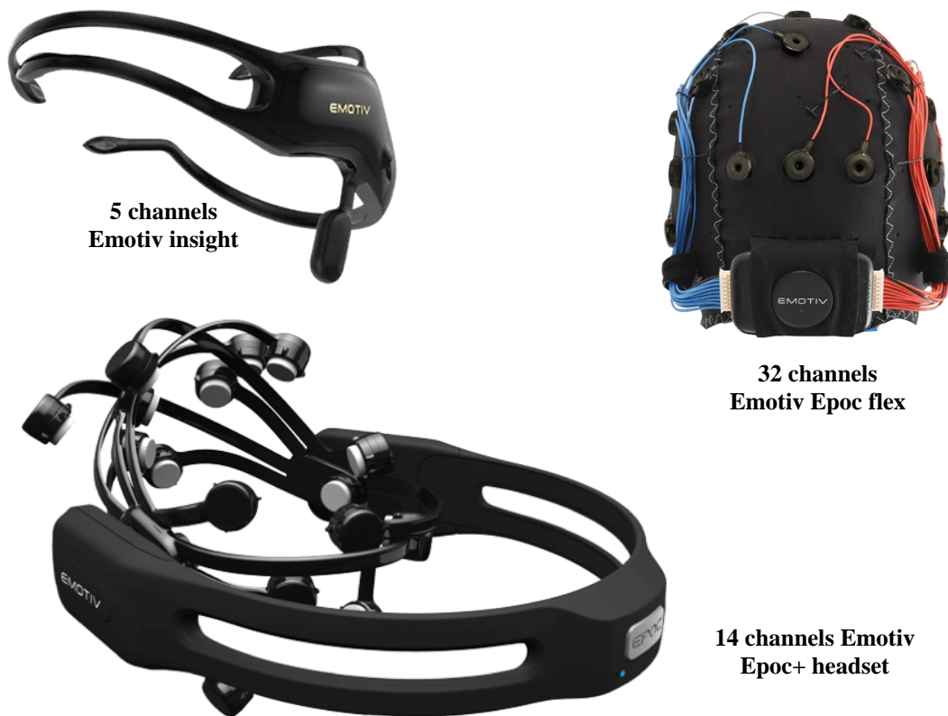
Figure 3.3: Emotiv Epoc EEG data recording equipment.
