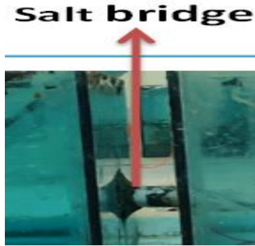
Figure 3.3 Photograph of the salt bridge for MFC
