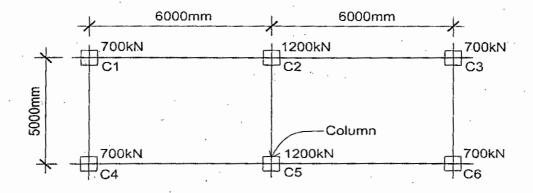
Design a continuous footing with foundation grade beam as shown in figure below. (35) All column sizes are 15"x15" and the allowable bearing capacity of soil is 1 tsf. Given:  $f'_c = 3000$  psi and  $f_s = 24000$  psi. Show the reinforcement details.
