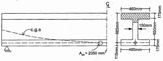
3. (a) Make a final design for the preliminary section as shown in figure, allowing  $f_b = -$  (15) 12.5 MPa,  $f_0 = 1035$  MPa. Other given values were:  $M_T = 435$  kN-m;  $M_G = 55$  kN-m;  $f_t = -11$  MPa;  $f_{se} = 860$  MPa and F = 826 kN.
