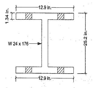
(b) Select the beam section by using 50 ksi steel and both the LRFD and ASD (20) methods. Select the lightest available section for the situation shown in figure. Bracing is provided only at the ends and at mid span.
