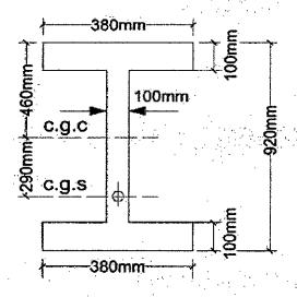
(b) Check the shear strength for the beam shown in figure at section 1-1 which is h/2 (20) from the support. Given that this section is adequate for  $W_u = 70 \text{ kN/m}$ ,  $A = 23.45 \times 10^4 \text{ mm}^2$ ,  $I = 2.304 \times 10^{10} \text{ mm}^4$ ,  $S = 5.12 \times 10^7 \text{ mm}^3$  and  $f_c' = 49 \text{ MPa}$ .
