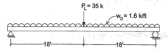
(b) Using both LRFD and ASD, select the most economical sections with F<sub>y</sub> = 50 ksi, (20) unless otherwise specified, and assuming full lateral bracing for the compression flanges as shown in figure. Working or service loads are given for each case, and beam weight is not included.
