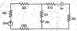
b) State Thevenin's theorem and by using the theorem, replace the following network with (13) reference to terminal AB.
