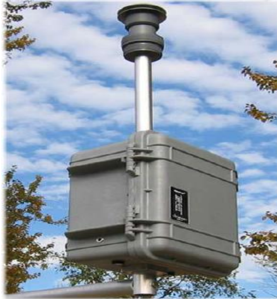
Figure-3.4: Mini Vol™ Tactical Air Sampler (TAS) is attached in Electric pole near administrative building for sample collection.
