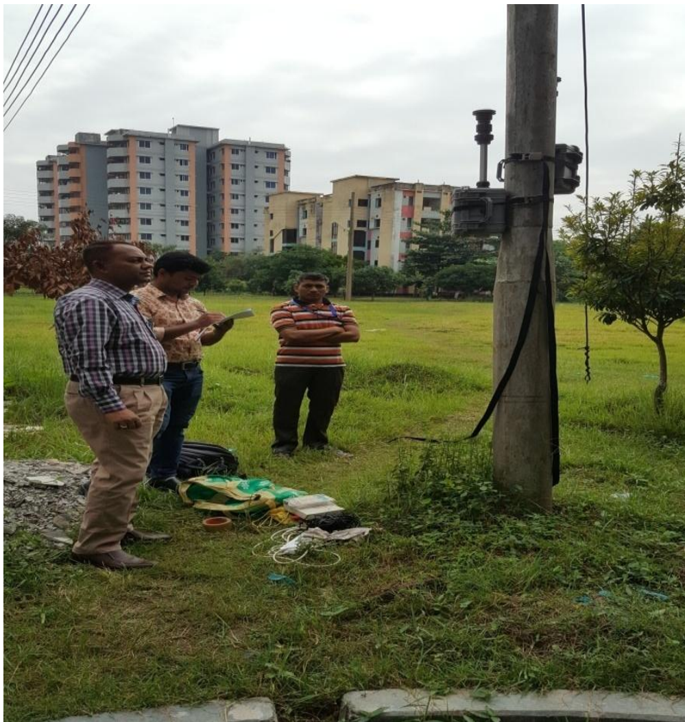
Figure-3.5: Taking reading from Mini Vol™ Tactical Air Sampler (TAS) at JUST campus.
