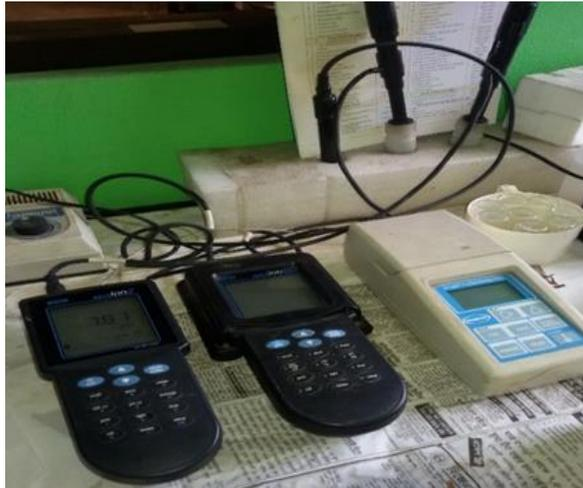
Photo 10: EC, pH and turbidity test
