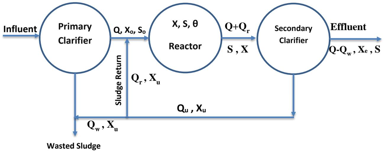
Figure 1: Process Flow diagram of activated sludge processing
