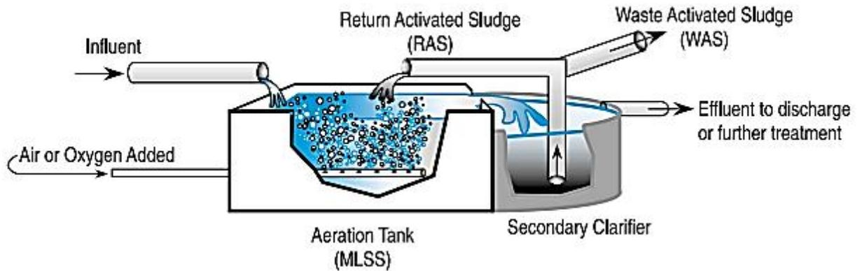
Figure 2.10: Basic schematic of the biological process in an activated sludge processing unit
