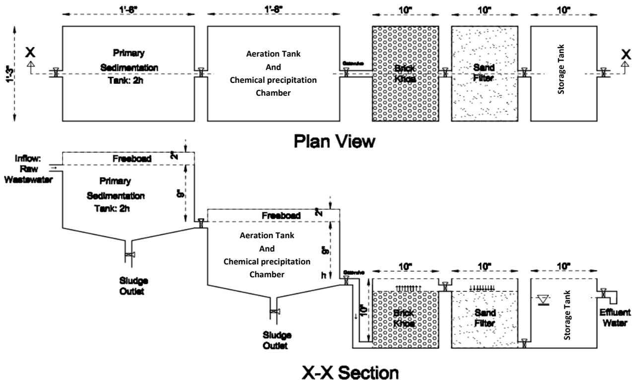
Figure 3.7: Instrumental setup and operation of developed treatment unit
