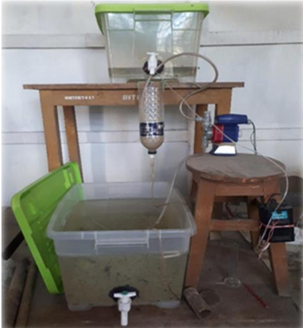
Photo 16: Laboratory Set-up of Activated Sludge Processing Unit
