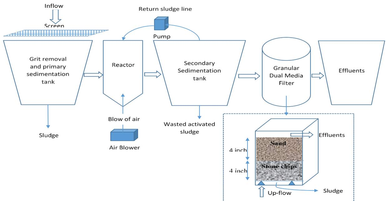
Figure 5.17 (a): Flow diagram of modified treatment plant
