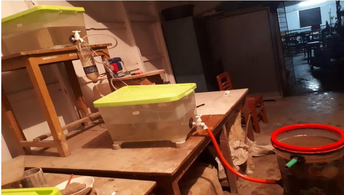
Figure 5.17 (b): Laboratory setup of modified treatment plant for municipal wastewater
