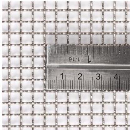
Figure 3.4: Bar screen of 5mm x 5mm in size steel wire mess
