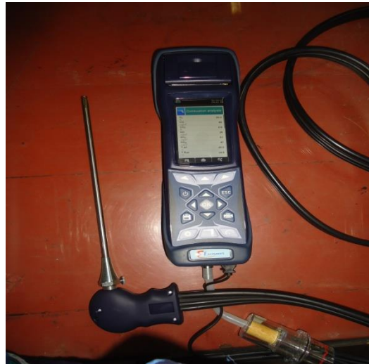
Figure 3.9 Industrial combustion gas analyzer
