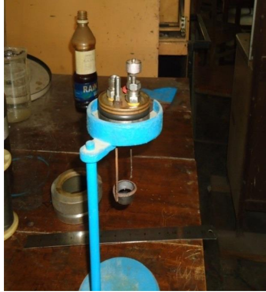
Figure 3.5 Connecting fuse weir with bomb
