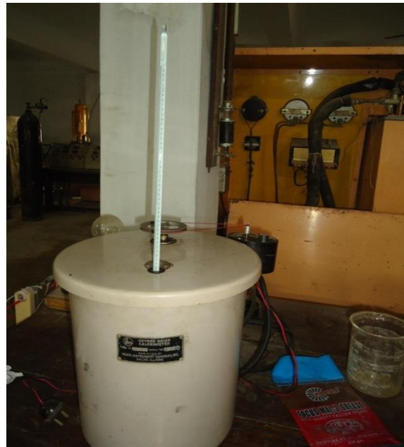
Figure 3.7 Final setting of Oxygen bomb calorimeter
