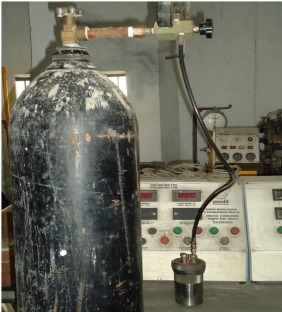
Figure 3.6 Oxygen supplying to the Bomb
