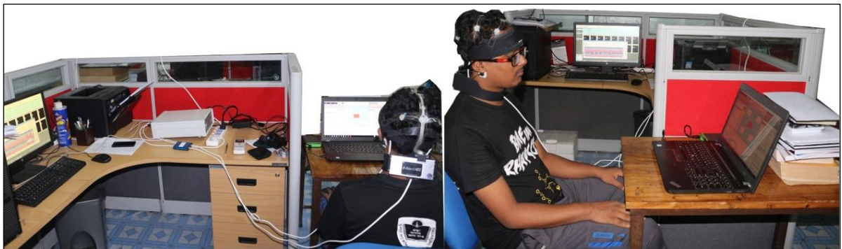
Figure 5.4: Data acquisition of voluntary and imagery movements by concurrent fNIR and EEG modalities.
