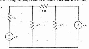
Find the current through 10  $\Omega$  resistor of the network as shown in the following figure -2(b).
