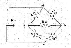
2(d). State Thevenin's theorem. Find the Thevenin's equivalent circuit for the network in the shaded area as shown in the following figure -
