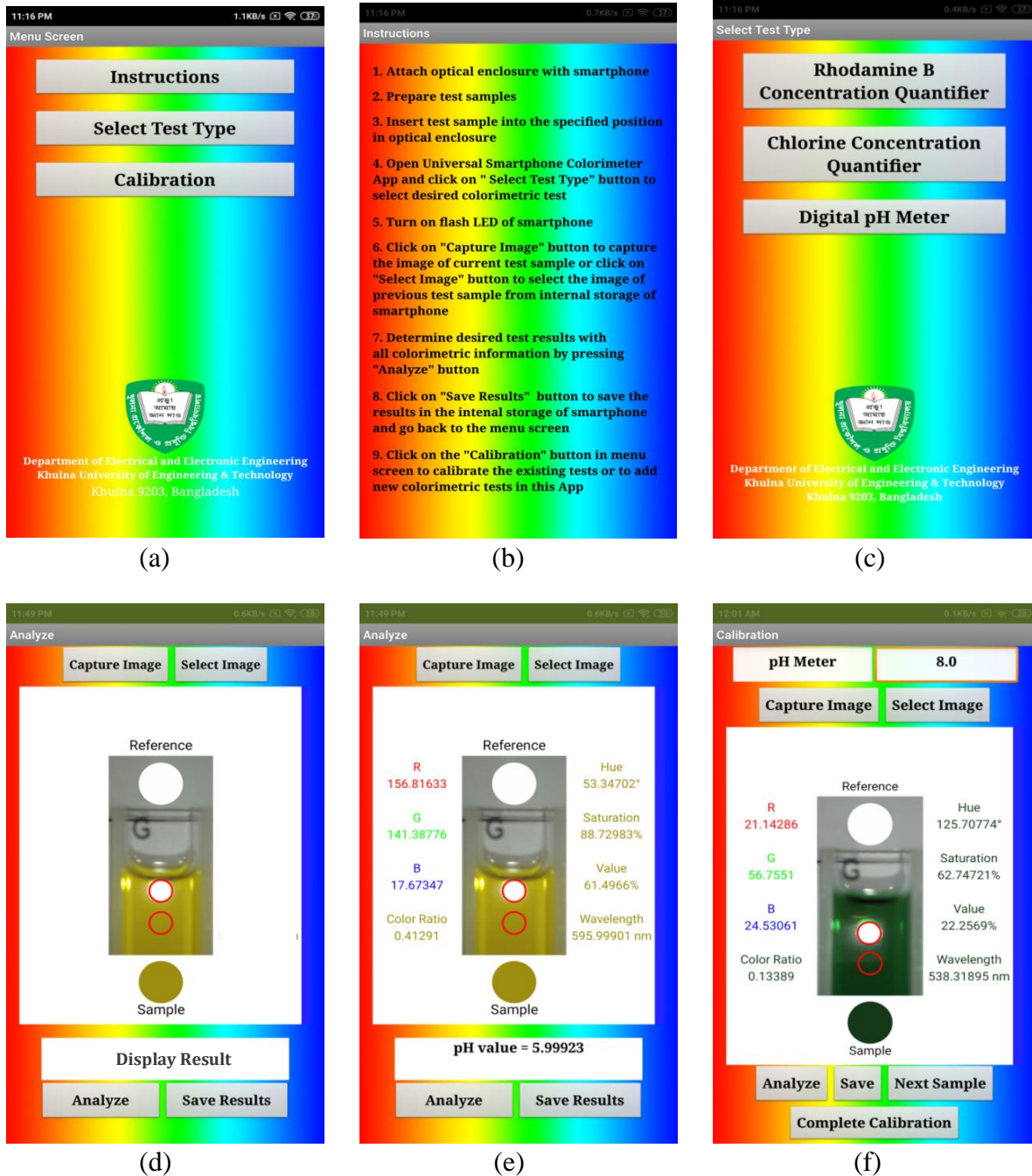
Fig. 3.4: Screenshots images illustrating the workflow of the customized Smartphone Colorimeter app: (a) menu screen, (b) instruction screen, (c) select test type screen, (d) selected or captured image of the test sample uploaded in analyze screen, (e) colorimetric test results and (f) the calibration screen.
